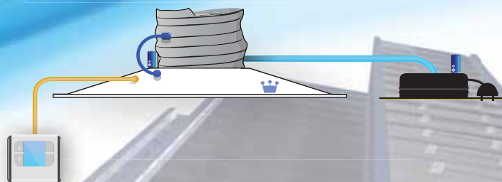
One diffuser with wall thermostat as master.
