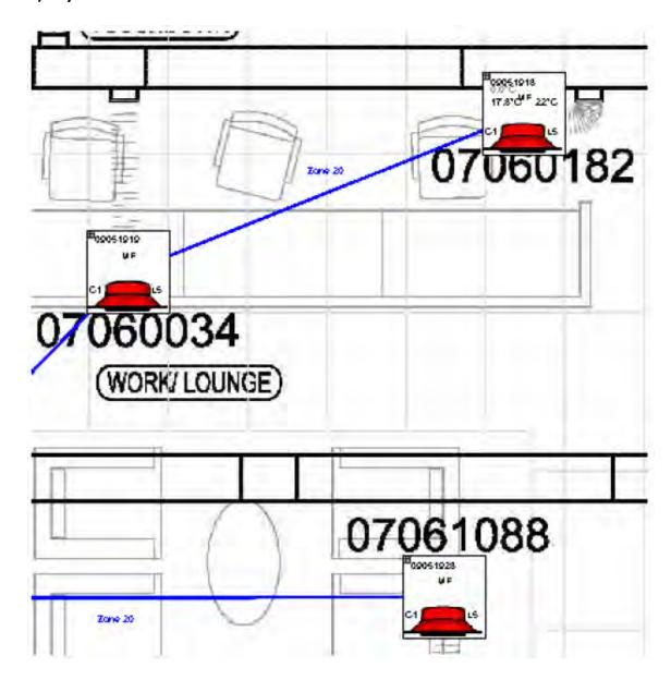
This view gives a graphical representation of the loop and zone relationships between the different diffusers on a diffuser network positioning each diffuser on a image background loaded using a project file.
