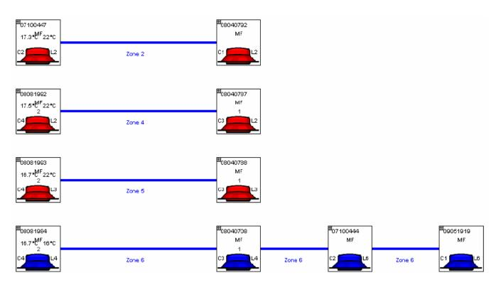
There can be up to 4 active channels. Each channel can have up to 15 diffusers where each diffuser have a specific channel and loop number assigned to it. To connect diffusers on different channels, the Zone concept is used. There are 60 possible zones.
