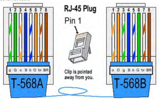
If connecting a PC to a Master Comms Unit through a switch or hub a normal straight-through cable can be used
