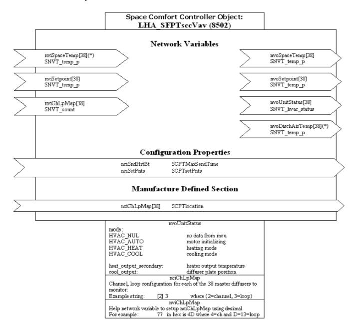
There are 38 functional blocks in the functional profile of the MCU Lon module that can be setup to bind with 38 master diffuser units on the MLM Proprietary network. The nciChLpMap configuration property string value (for example [2] 3) can be changed from the default value by using network tools like LONmaker.
