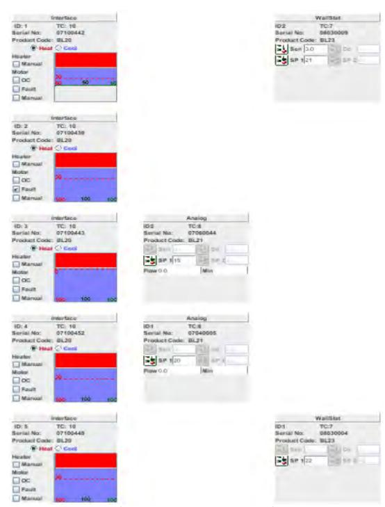
This view gives a graphical display of the relationships between the interface, analogue and wall stat modules of a diffuser network. Starting from the top of the screen, all the different channels are listed apart from each other. For example, using a TCP/IP connection there may be more than one channel grouping while a USB connection will always have only one channel.
