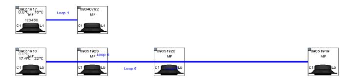
For a USB connection there is only one channel with 15 possible diffusers and only make use of the loop concept.
